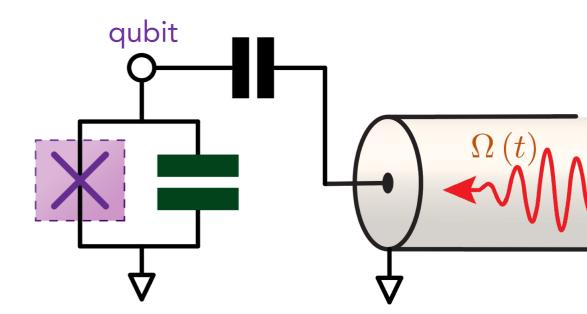
Qubits: Nonlinear quantum oscillator Gates: coupled microwave pulses
